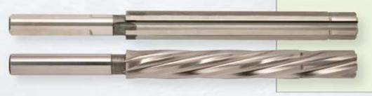
Type "L" long series pilot reamers have a standard total length of 6" (150mm) with 4" (100mm) Flute length and are designed to produce larger diameter close tolerance holes or for longer reach applications.
